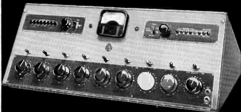
BC-2B STUDIO CONSOLETTTE. "Low-boy" console offers deluxe, operation-proved features usually found in custom-built equipment—but at a standard "package" price. Includes complete high-fidelity speech input provisions for 2 studios, announce booth, 2 turntables, 5 remotes, and network.
